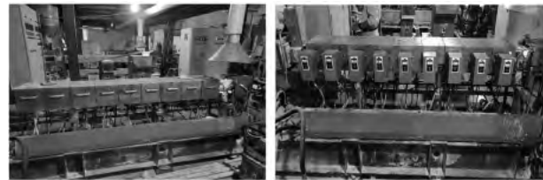
(a) Schematic diagram of the original resistance heating coil (b) Schematic diagram of electromagnetic heating coil
