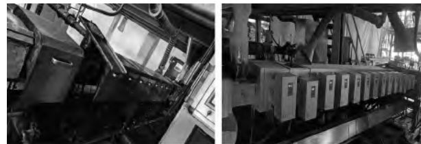
(a) Schematic diagram of the original resistance heating coil (b) Schematic diagram of electromagnetic heating coil
